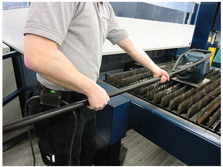
Off switch on the cable
