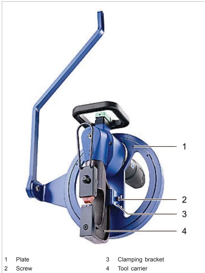
TruTool TF 350 with installed slewing ring
